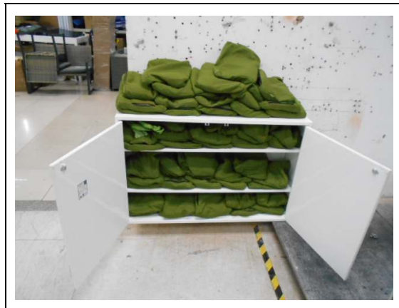
Wall Mounted Cabinet Load Test
