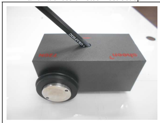
Paint Hardness on Steel Test Set-up
