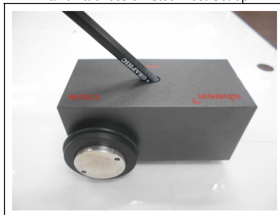
Paint Hardness on Steel Test Set-up
