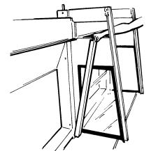
12. Remove from carton and install front sill. Make sure sill engages screw and washer located underneath each side panel end, then fasten each sill end to a side panel using one screw on top of sill through hole in tab of side panel.
