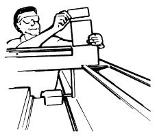
19. Remove from carton and install front panel(s) in the slots provided for the tabs.
