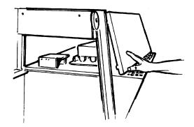
21. Replace weight side panels. Check hood - it should be square and plumb.
