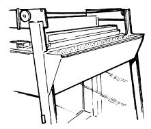
20. Remove from carton and install top panel(s) in slots provided for tabs. For safety purposes, fasten center angle with screw.
