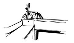
11. Install pipe chase assembly to hood. Fasten using supplied screws and plastic caps.
