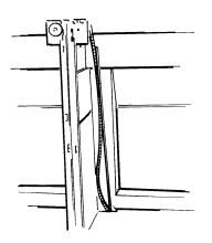
9. Install side panels. Top of panel should fit into outer slot. Bottom of panel slides over plenum tab. All panels must rest flush on work surface.
