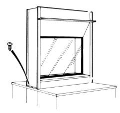
5. Remove pulley bracket assembly from both ends. Raise weight pan/cable assembly to top of hood and lock in installation position.
