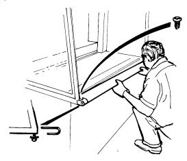
Install top panel and light assembly to top of hood. Slide top panel into extrusion at rear of hood. Make sure top panel is in extrusion, if not, gently pound into place with a rubber mallet.
