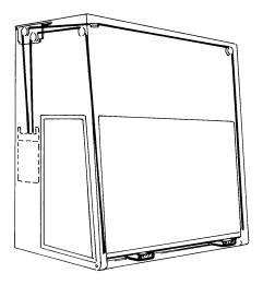
15. Remove counterweight shipping tape. Engage angle on counterweight with angle of sash pull.
