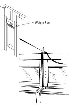
6. Remove from carton and install both right and left upright bracket assemblies.
