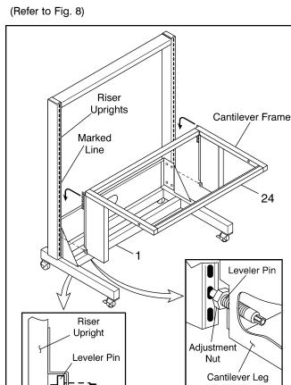
1. Cantilever shelves are shipped in two parts consisting of a frame assembly and top. All mobile cart frames must be fully assembled and leveled before tables or shelves are attached.
