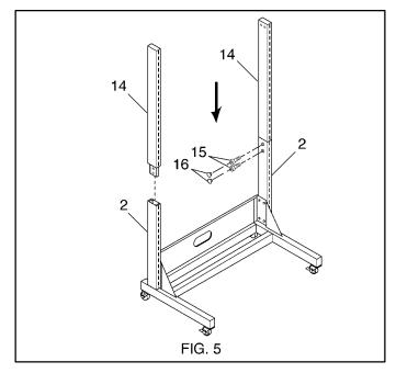
3. Locate the socket screw caps (16) and firmly press one cap into the center of each cap screw head (15).
