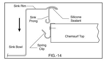
Carefully position the sink into the cutout so that the downward prong rests on the spring clips.
