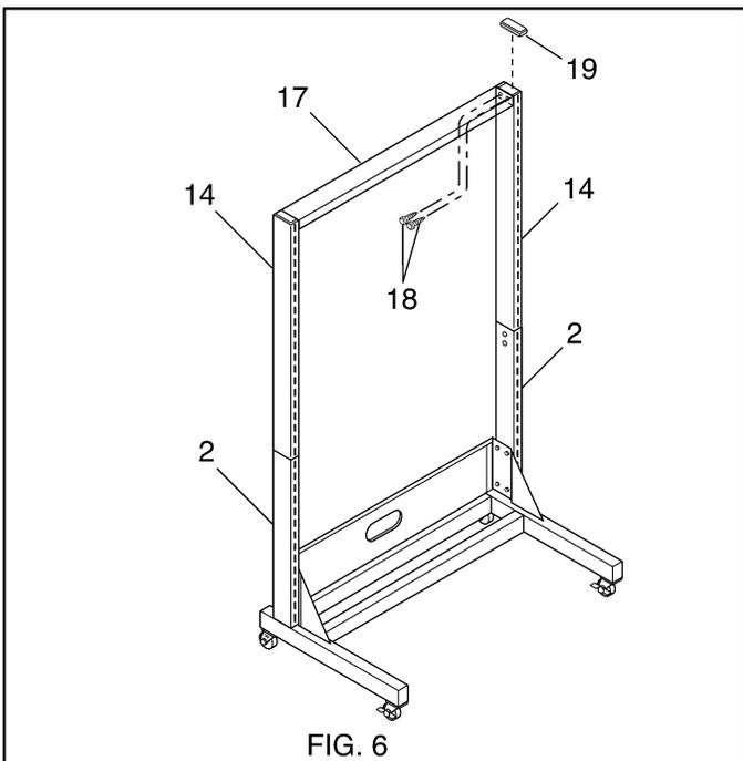
4. Locate the upper cross rail (17) and position it at the top and between the two upper riser assemblies (14) previously installed.
