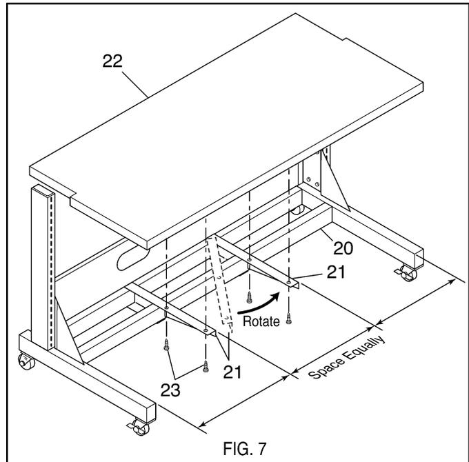
2. Place each shelf bracket (21) at approximately a 45° angle between the lower frame braces and rotate into place perpendicular to the frame bracing. The top and bottom flanges of the shelf brackets should slide over the top and bottom of the frame braces locking the brackets in place. Allow equal spacing between shelf brackets and lower frame ends.
