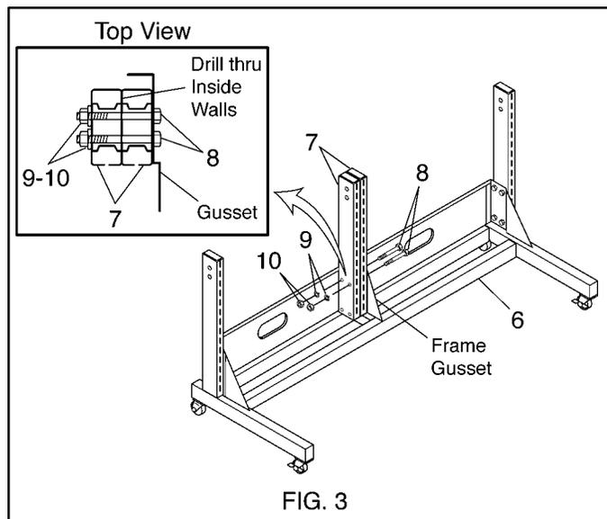
5. When attaching double riser uprights to wider frame assemblies, it will be necessary to drill holes through the two inside riser walls.
