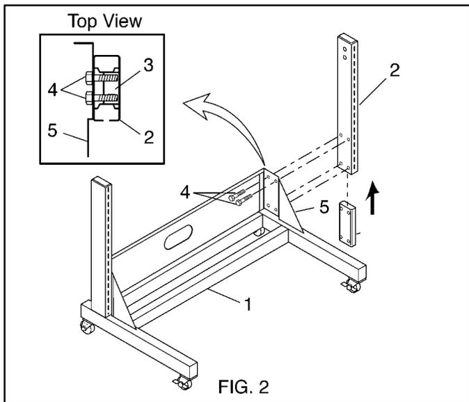
3. Orient the riser uprights (2) with the adjustment slots facing to the front.
