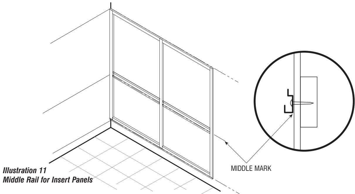
6. Insert and attach the vertical rails with four No. 10 flat-head screws starting with a single member at the corner. Note: The top and bottom rails are notched on six-inch centers, to ensure proper system modularity. Measure over the desired number of feet and insert a single- or double-slotted upright, or core support panel as required and continue this process until the set up is complete.
