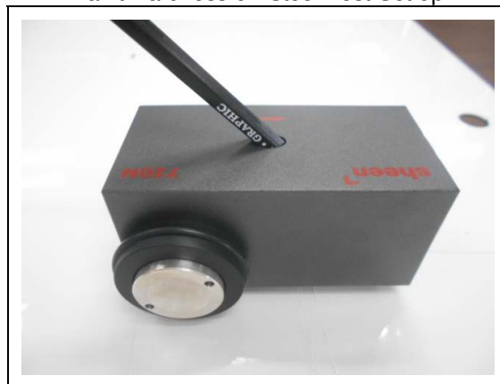
Paint Hardness on Steel Test Set-up
