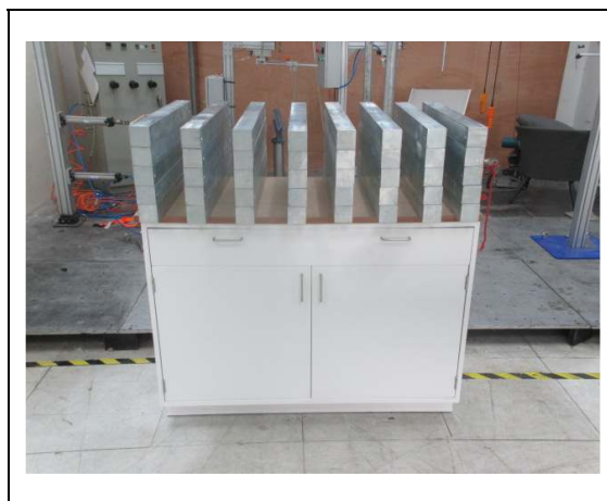
Cabinet Load Test
