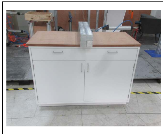
Concentrated Load Test
